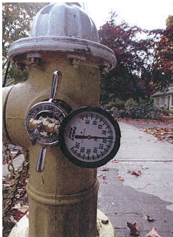
Residual hydrant: residual pressure reading
