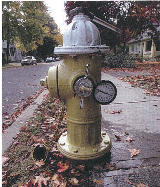
Residual hydrant: residual pressure reading
