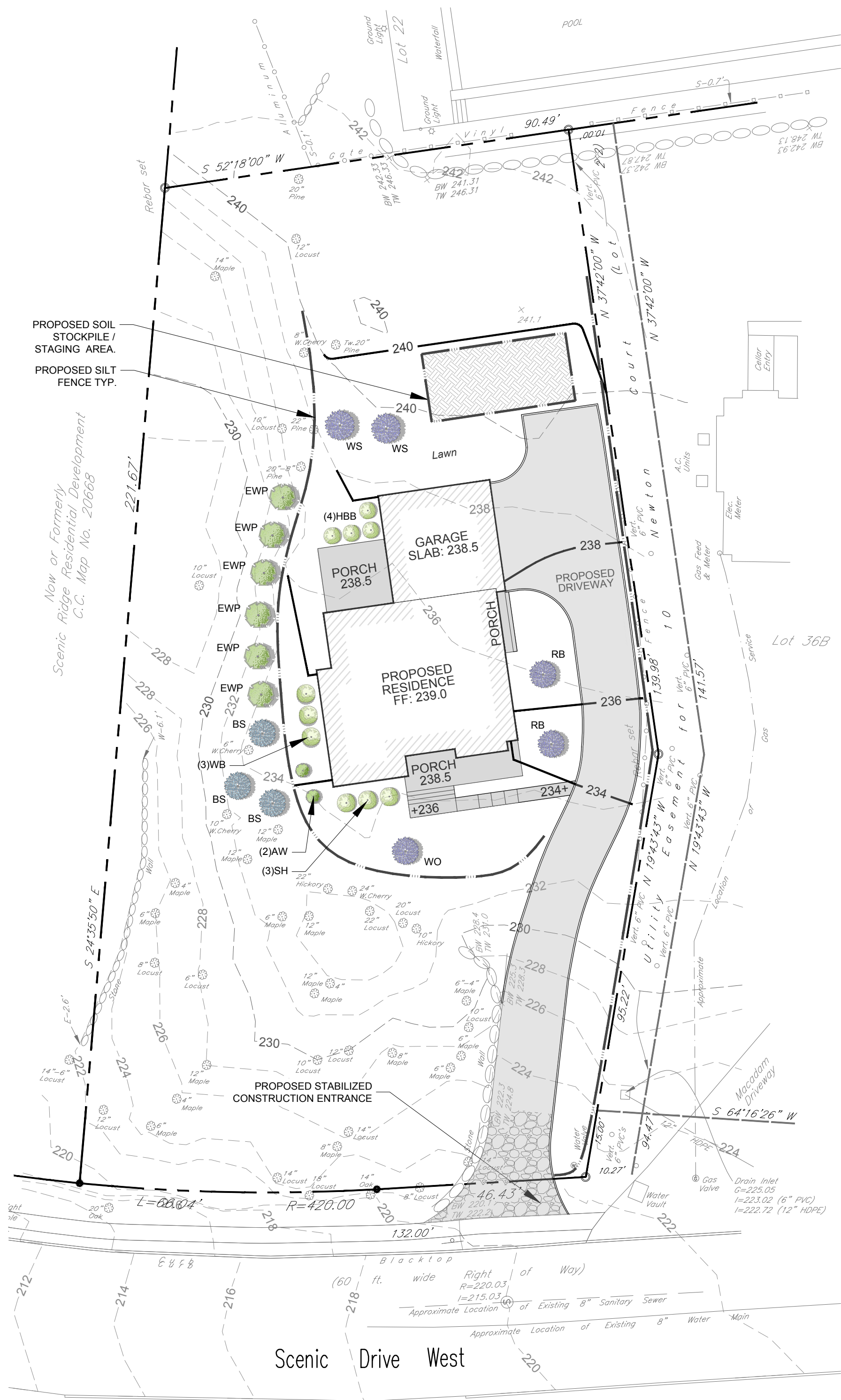
EROSION AND SEDIMENTS CONTROL PLAN SCALE: 1"=20'
