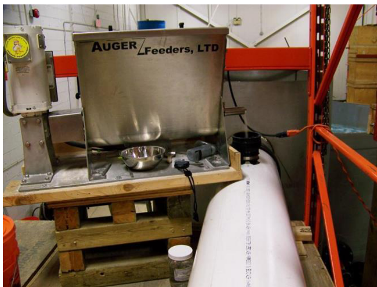
Figure 7 Sediment Auger Feeder
