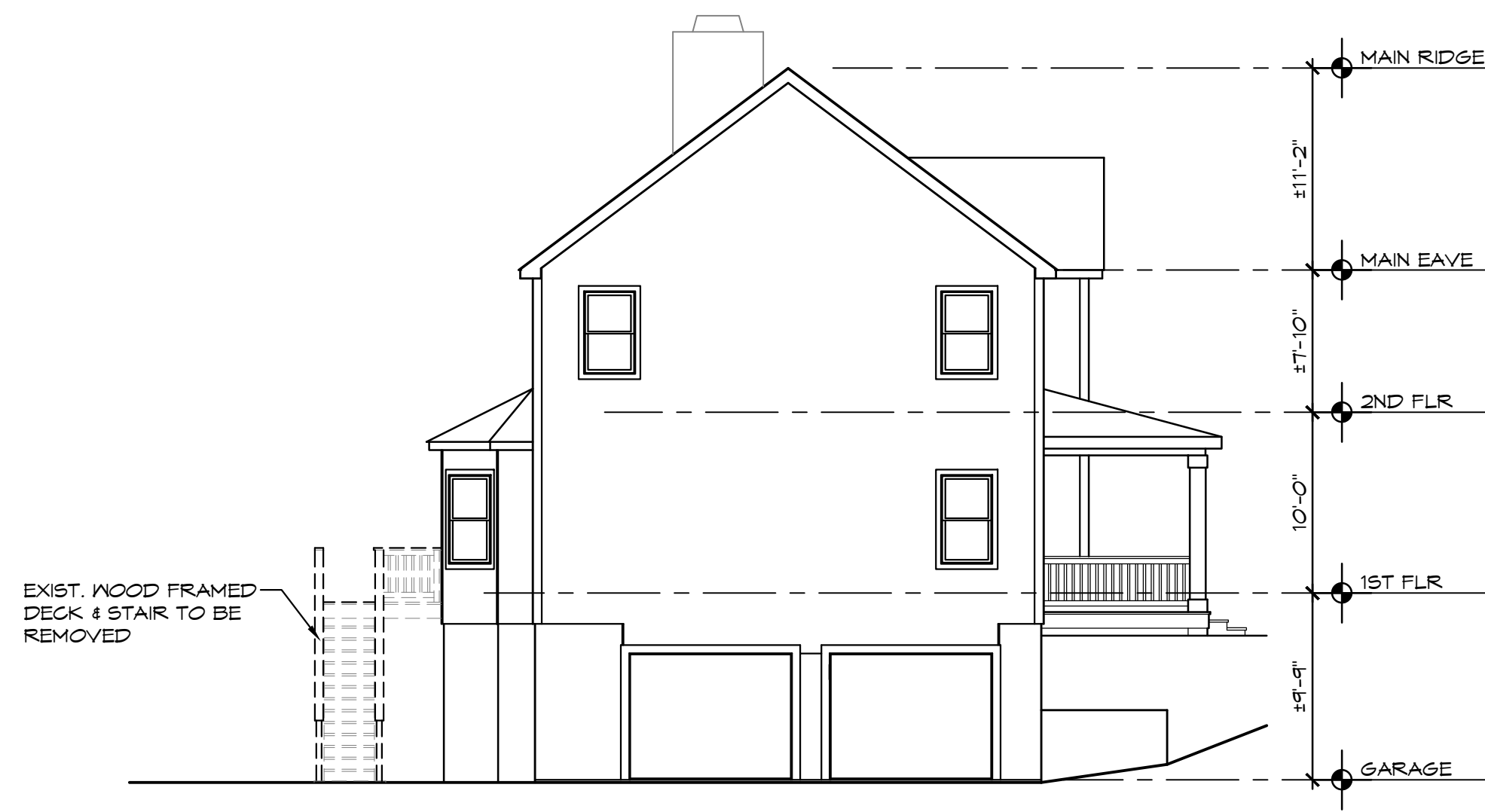
3 SOUTH ELEVATION WITH DEMOLITION 1/8" = 1' - 0"
