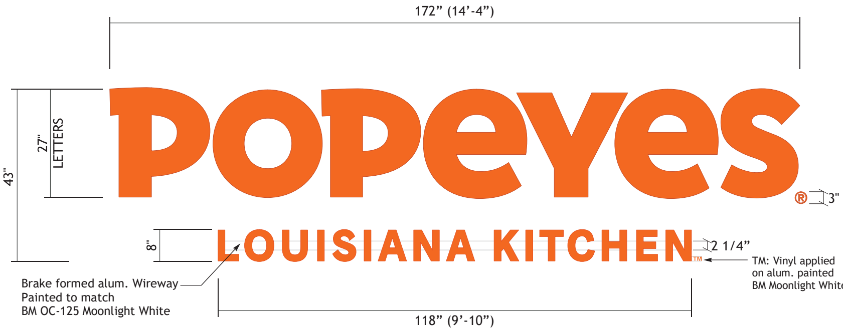
N1 ILLUMINATED CHANNEL LETTERS AREA: 52.55 SQ FT SCALE: 1/2" = 1'-0" FRONT VIEW SIDE VIEW SCALE: 1/2" = 1'-0"
