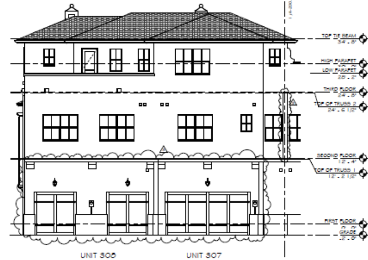
PARTIAL REAR ELEVATION 3/16" = 1'-0"
