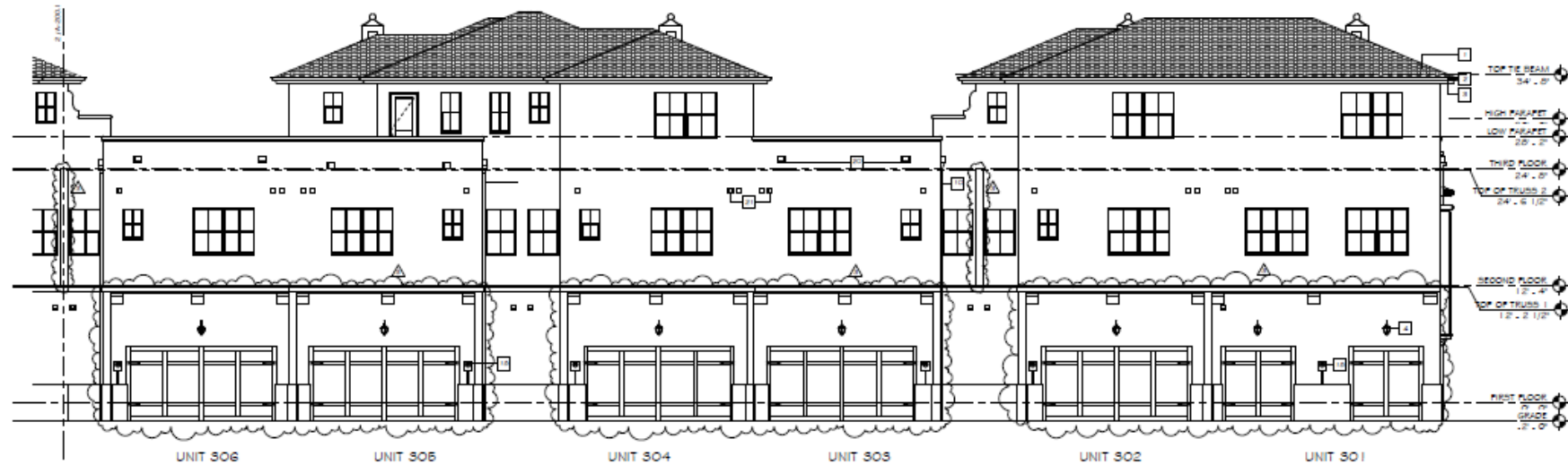
PARTIAL REAR ELEVATION 3/16" = 1'-0"
