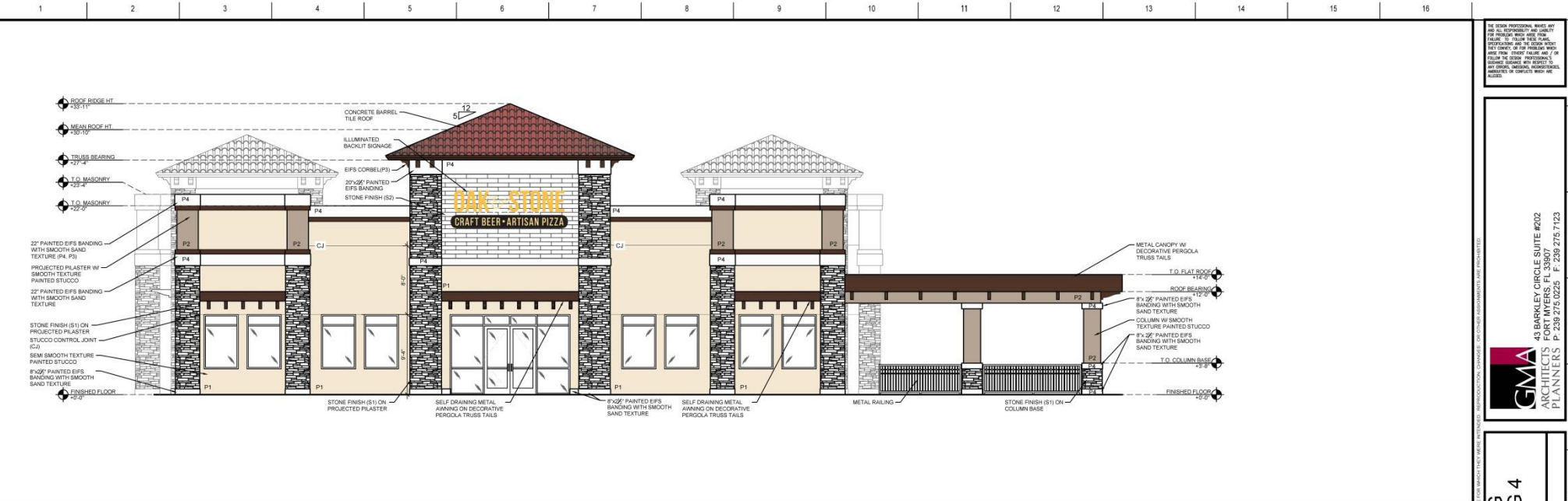
G1 WEST EXTERIOR ELEVATION - ENTRY SCALE 3/16" = 1'-0"
