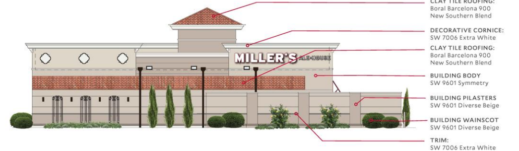
REAR ELEVATION: Scale: 3/32"= 1'-0"
