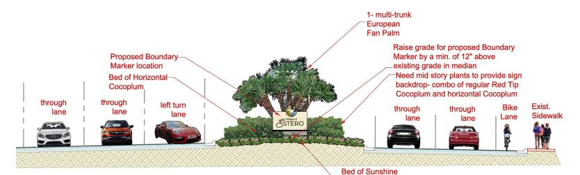
Cross Section of Proposed North Boundary Marker on Three Oaks
