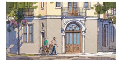
Multi-pane, wooden windows and doors
