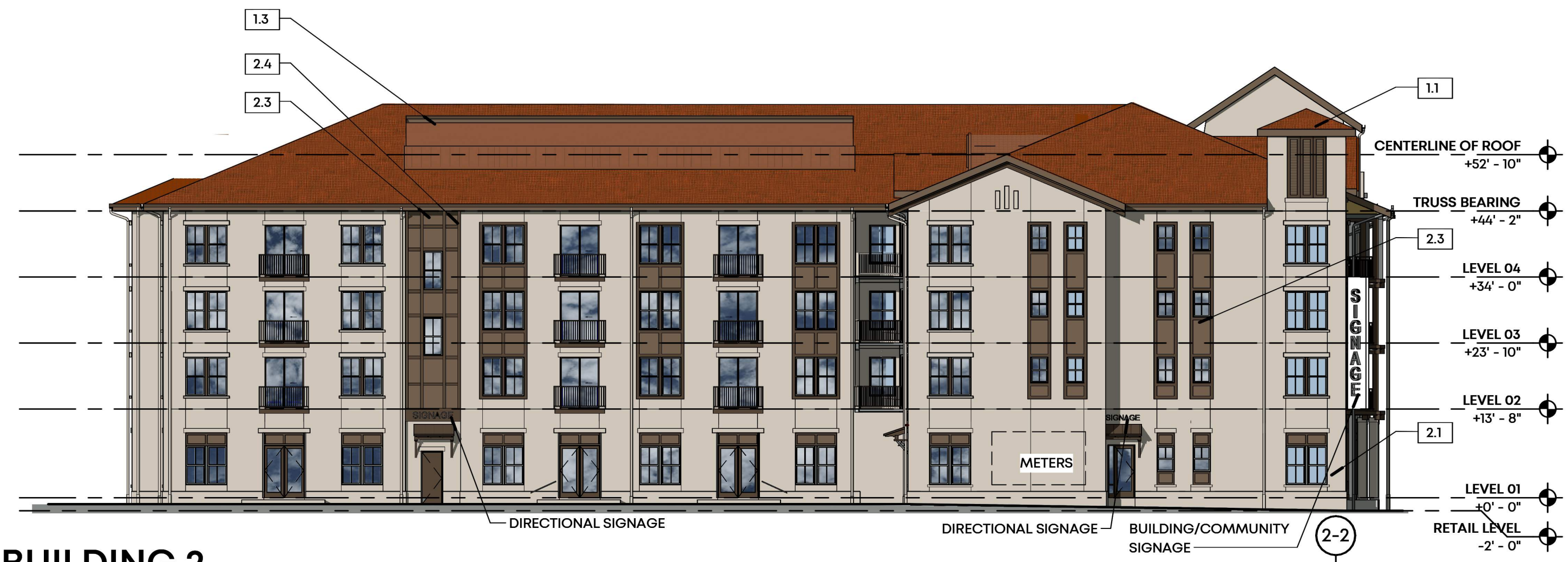
11 EAST ELEVATION - BUILDING 2 SCALE: 1/16" = 1'-0"
