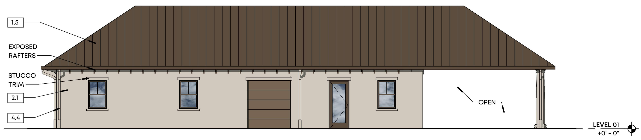
6 SIDE ELEVATION - MAINTENANCE BUILDING SCALE: 1/8" = 1'-0"
