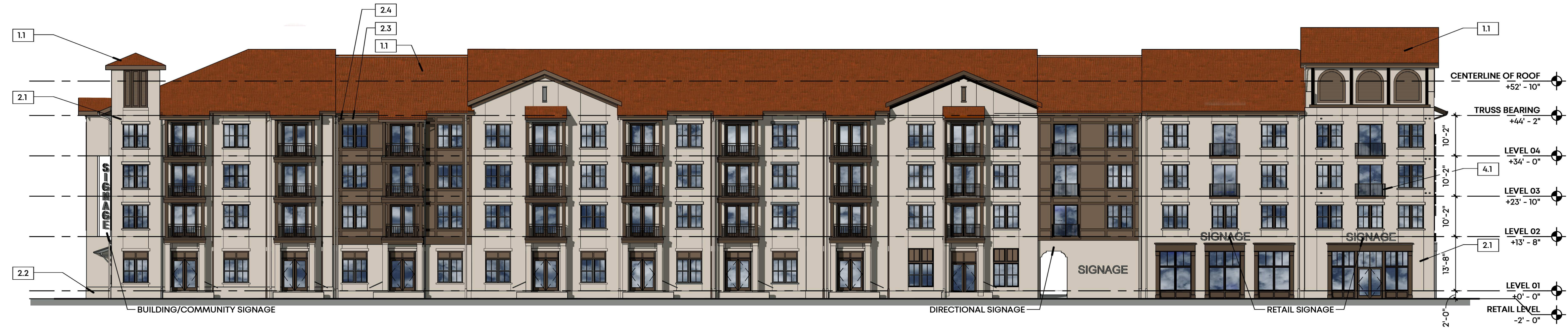
1 NORTH ELEVATION - BUILDING 2 SCALE: 1/16" = 1'-0"
