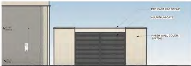
1 COMPACTOR ENCLOSURE - ELEVATION 1 5/8" = 1'-0"
