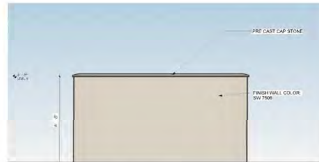
2 REFUSE ENCLOSURE A & B - ELEVATION 2 1/2" = 1'-0"
