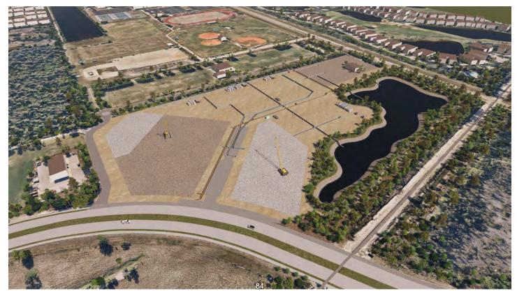
4. Installation of the base material for the parking area. This would allow these areas to be used for staging of any material needed to complete the construction of the proposed developments.
