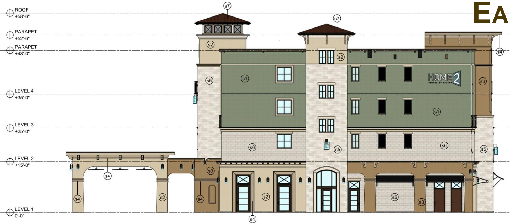
EAST BUILDING ELEVATION (RIGHT) SCALE: 1/8" = 1'-0"
