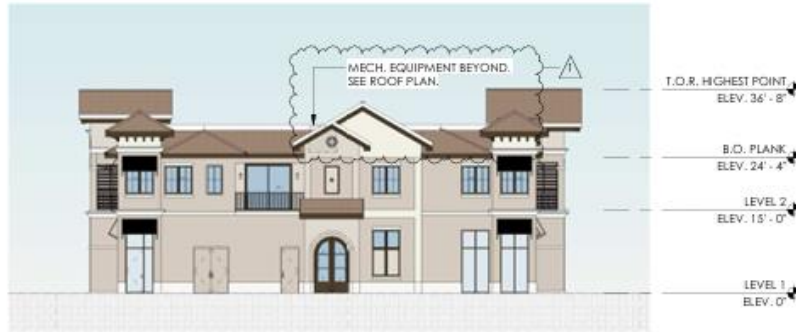
1 BUILDING C WEST ELEVATION SCALE: 1/16" = 1'-0"
