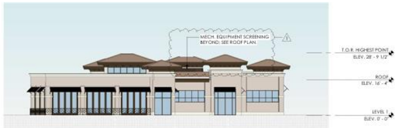
④ BUILDING C1 WEST ELEVATION SCALE: 1/16" = 1'-0"
