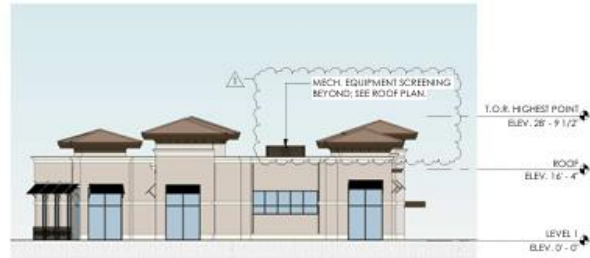
③ BUILDING C1 SOUTH ELEVATION SCALE: 1/16" = 1'-0"
