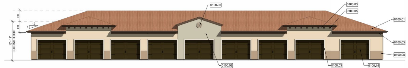
Front & Rear Elevation 18-Bay Garage
