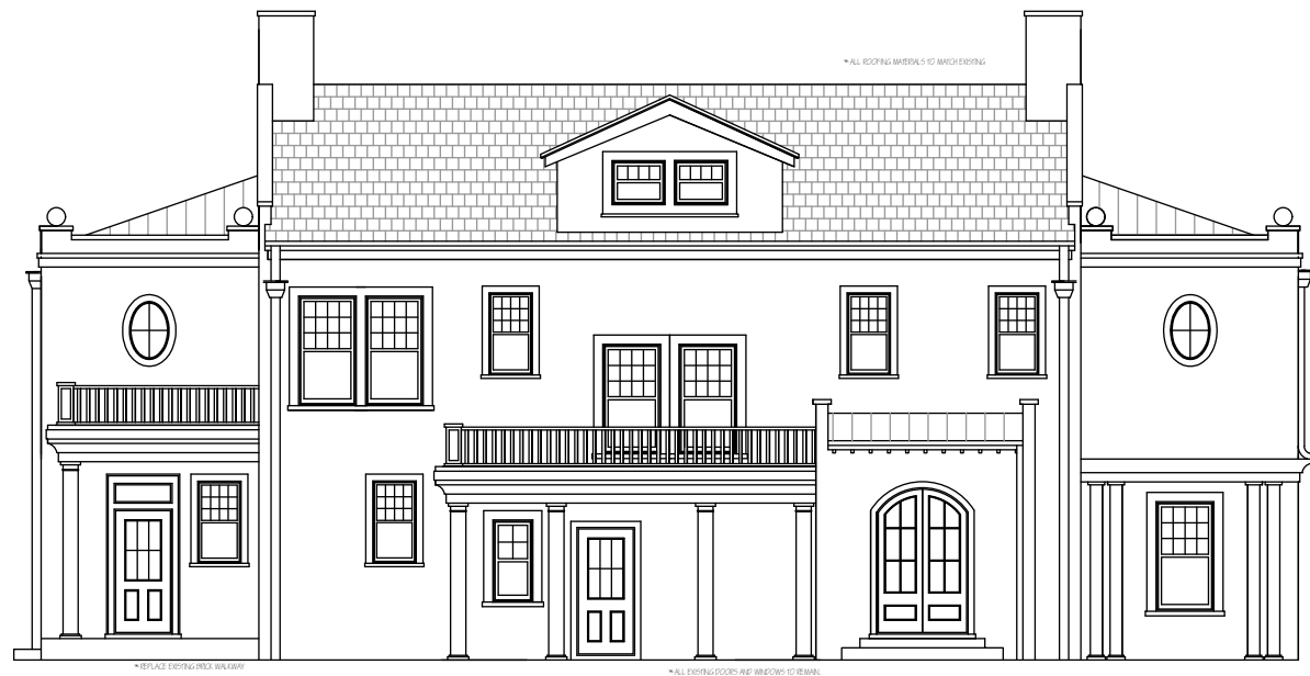
4424 SHEPARD PLACE - REVISED REAR ELEVATION SCALE \frac{1}{8}" = 1'
