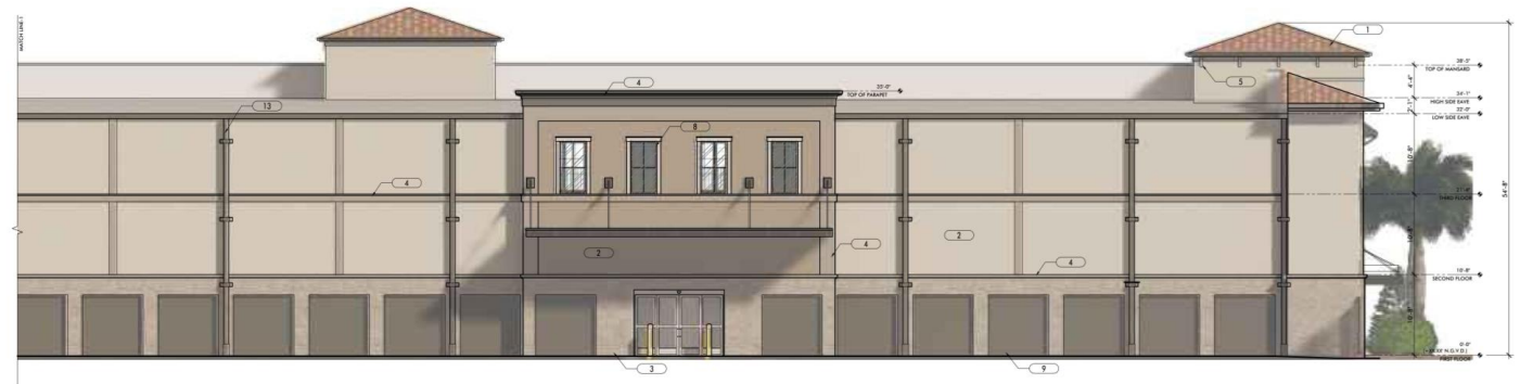
STORAGE BUILDING - NORTH ELEVATION 1/8" = 1'-0"
