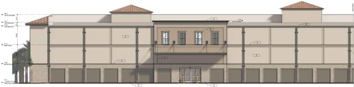
STORAGE BUILDING - NORTH ELEVATION 1/8" = 1'-0"
