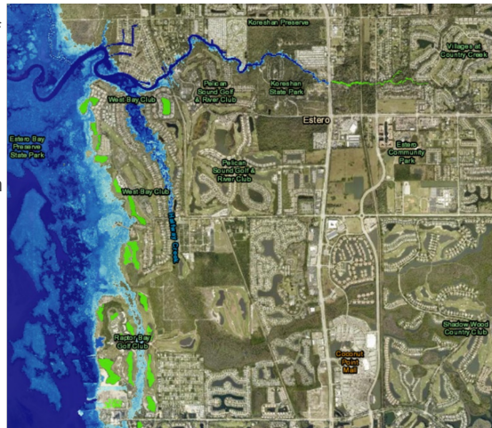
Figure 4-4 3-feet of Sea Level Rise Extent in Village of Estero (Data Source: NOAA Sea Level Rise Viewer). Estero River is tidally influenced and may let sea level rise impacts reach inland up to S Tamiami Trail (US 41) and residential areas such as Villages at County Creek
