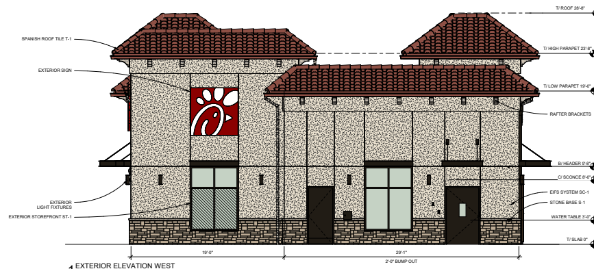
1 EXTERIOR ELEVATION WEST 14'-0" x 14'-0"
