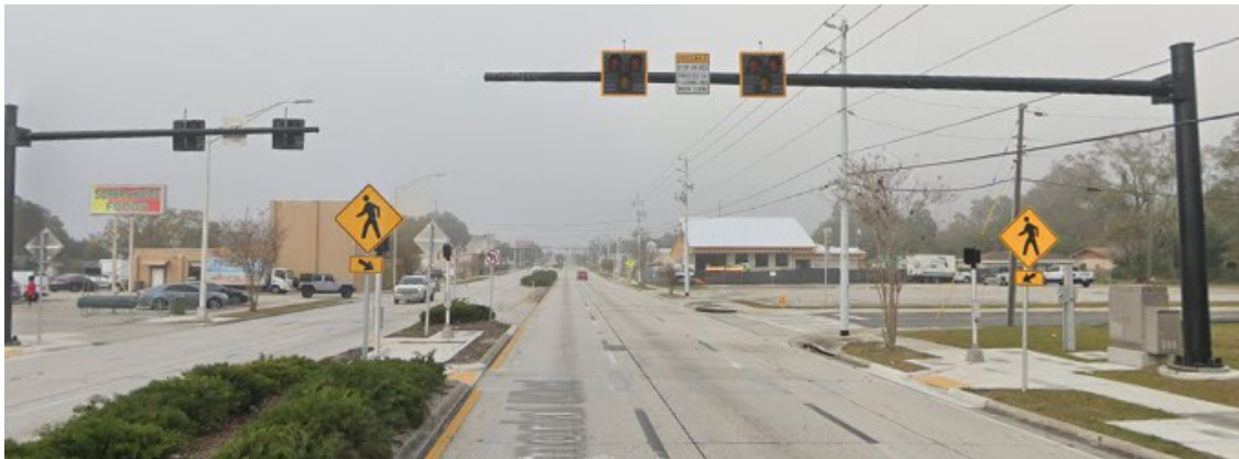
PEDESTRIAN HYBRID SIGNAL (HIGH INTENSITY ACTIVATED CROSSWALK – HAWK)
